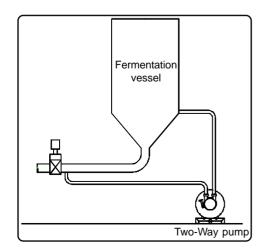
The TWO-WAY can pump in either direction. 1) *Product recirculation.*
